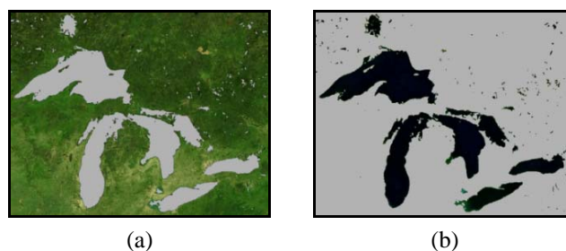
Figure 11. Result of region extraction algorithm applied to the geo-image obtained in the analysis stage for the geo-image 3.
